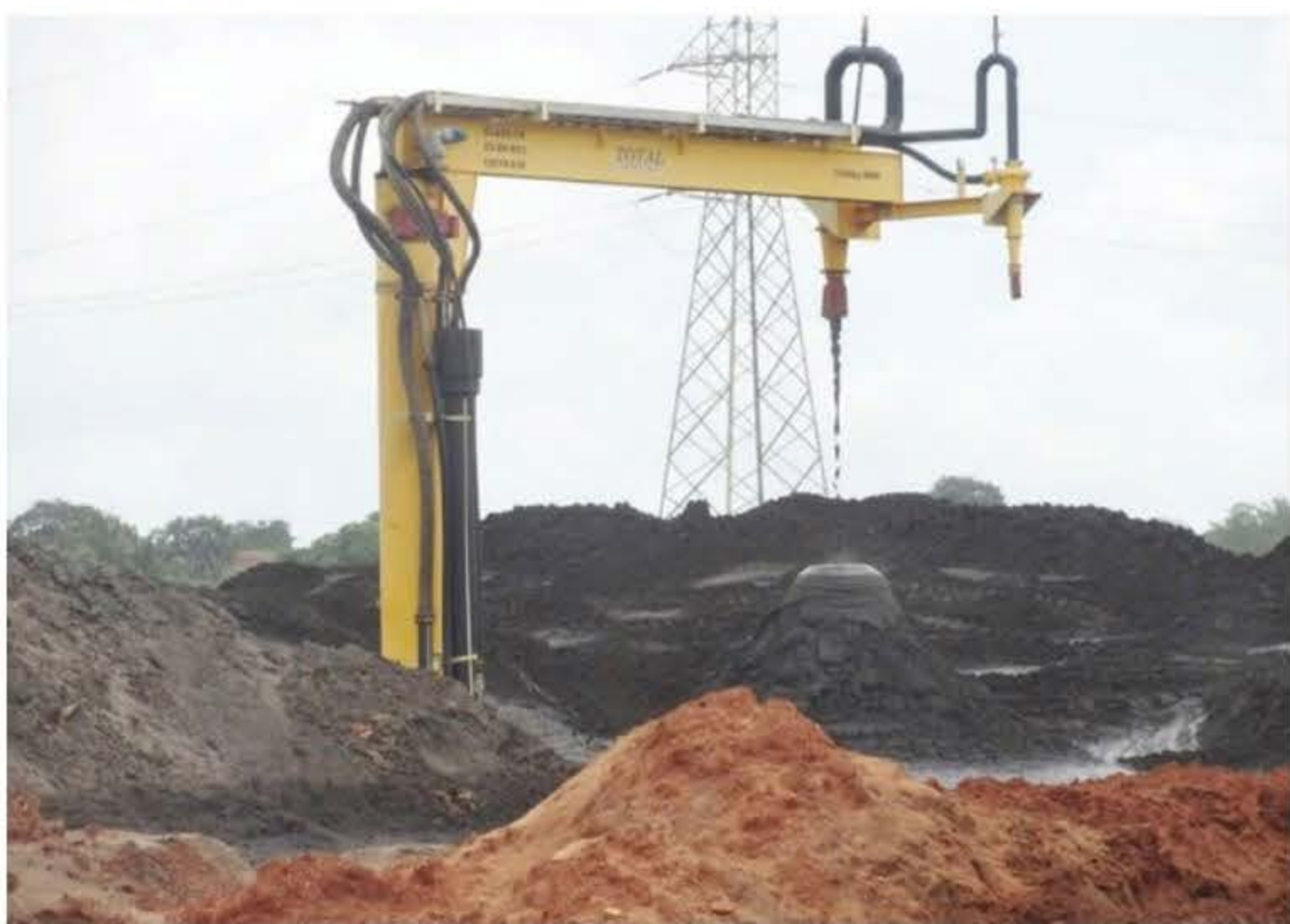
The tailing stacker separating the minerals from the soil at a titanium mining base in Kwale on September 17, 2014. FILE PHOTO | NATION MEDIA GROUP
